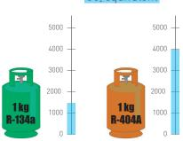
Therefore, the HFC phase-down hits HFCs with a high GWP, such as R-404A and R-507A, hardest; and if the consumption of these HFCs does not go down rapidly, all other HFCs, including blends containing HFCs, will suffer as a result.
